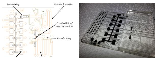
**Figure 1. Schematic and image of SynBioChip for automating: combinatorial gene mixing, assembly, electroporation, cell culture and assay.**
