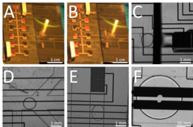
**Figure 3. Digital microfluidics is initially employed for the on-demand generation and merging of droplets containing DNA and ligation reagents (A,B). Vacuum actuation allows transfer of droplets to a polydimethylsiloxane channel (C) where fluorinated oil is pumped to move droplets through the device (D). Channel electrodes allow merger of droplets containing cells with assembled plasmid (E). Genes are delivered by electroporation with 1800 V/cm pulses (F).**
