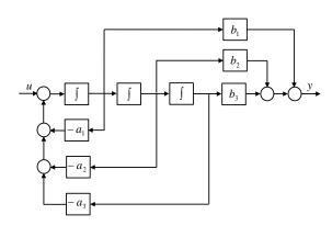
Figure 1: A physical realization of the LTI system  $H: u \mapsto y$  defined by the transfer function given by (1). The circles denote the summation junctions.
