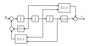
Figure 2: A sample block diagram illustrating a physical realization of the class of nonlinear systems of interest to us. The nonlinearities  $f_1$  and  $f_4$  can be Hill-type or power nonlinearities whereas  $f_2(x,y) \doteq xy$  and  $f_3(x,y) \doteq f_i(x)f_j(y)$  where  $(i,j) \in \{(1,1), (1,4), (4,1), (4,4)\}$ .
