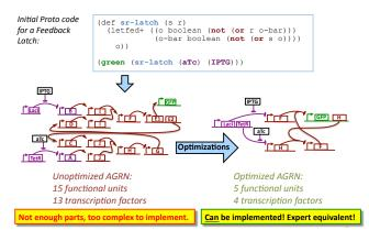
Figure 3: A high-level program is compiled to an AGRN and then optimized.
